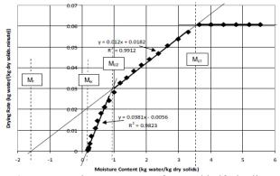
**Figure 7.** Drying rate curve of green kiwifruit slices with an air velocity of 0.20 m/s at ambient humidity and temperature of 80°C for replication 2 of green kiwifruit (Data 4) showing the FRP drying coefficients regressions, critical moisture contents, residual moisture content and dynamic equilibrium moisture content;  $M_{c2}$  = second critical moisture content;  $M_r$  = residual moisture content;  $M_e$  = dynamic equilibrium moisture content).
