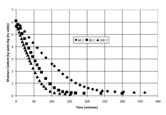
**Figure 3.** Representative drying curves of gold kiwifruit slices with an air velocity of 0.20 m/s at ambient humidity and different temperatures.
