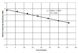
**Figure 6.** Drying curve of green kiwifruit slices with an air velocity of 0.20 m/s at ambient humidity and temperature of 80°C for replication 2 of green kiwifruit (Data 4) showing the CRP drying rate regression.
