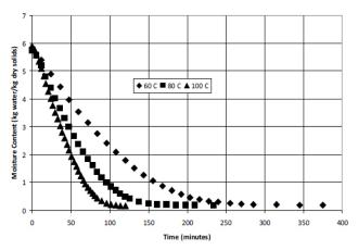
**Figure 2.** Representative drying curves of green kiwifruit slices with an air velocity of 0.20 m/s at ambient humidity and different temperatures.
