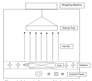
**Figure 1.** Schematic diagram of the hot air dryer used in the experiments.
