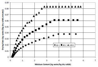
**Figure 4.** Representative drying rate curves of green kiwifruit slices with an air velocity of 0.20 m/s at ambient humidity and different temperatures.
