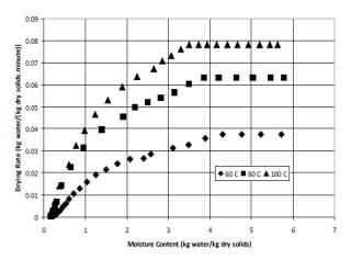
**Figure 5.** Representative drying rate curves of gold kiwifruit slices with an air velocity of 0.20 m/s at ambient humidity and different temperatures.
